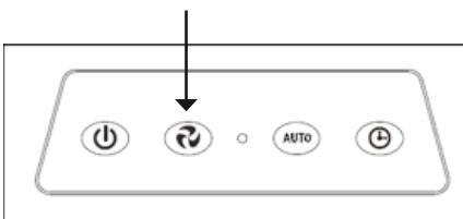
Press the speed options button for 3 seconds to reset the filter timer.
